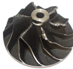
Pitting on the compressor blades
