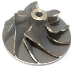
Chipping to the compressor blades
