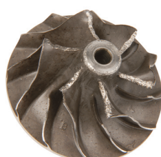
Damage to inducer of turbine wheel
