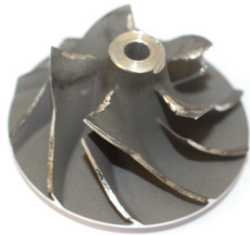
Chipping to the compressor blades
