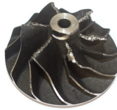
Pitting on the compressor blades
