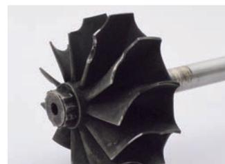
Turbine wheel failure through HCF
