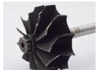
Turbine wheel failure through HCF
