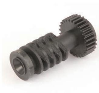
Worm gear failure due to restricted VNT mechanism
