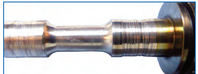
Scoring to journal bearing diameter of shaft wheel
